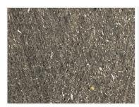
Asbestos-free, pressed composite friction material containing metallic components. AB3080 is based on phenolic resins with NBR ruber bonding system, containing short fibers, organic components, friction modifiers, metallic particles and fillers. AB3080 is suitable for dry and oil-immersed applications. AB3080 is not abrasive to the counter face material and is silence in operation, It is resistant to high pressures and has low wear rate even at high temperatures.
