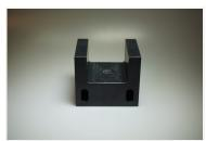
PET is a partly crystalline thermoplastic Polyester based on Polyethylene-Terephthalate. This material features outstanding dimensional stability as it is virtually unaffected by ambient moisture. A low coefficient of friction and excellent wear resistance combined with low creep and high E-modulus of elasticity in tension makes it the choice material for moving parts. Hot water resistance is low but it has better resistance to acids than Nylon or Acetal.
