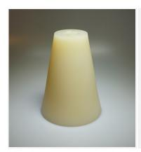
AE202HV is an unreinforced, high viscosity Polyamide 6. It has a higher impact resistance also at very low temperature, AS202HV does not break at room temperature during the Charpy impact strength test, the notched test has a value of 70 kJ/m².
