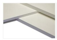
Mineral bonded steam-hardened calcium silicate board with a low volumetric mass that is resistant to moisture. This plate is mainly used for the realization of fire resistant electro cable ducts, ventilation and smoke extraction ducts and ducts for fire resistant pressure relief systems. Suitable for a wide range of applications in indoor environments.
