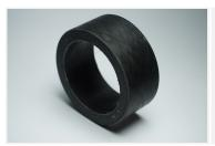
ASN116 is a composite bearing material for medium to high load and high temperature applications. It contains high-strength, continuously wound fibres encapsulated in an internally lubricated, high-temperature filled epoxy resin. ASN116 possesses good shock resistance, excellent chemical resistance, low friction and good anti-wear properties.
