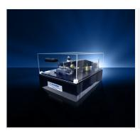
In accordance with ISO 7148, ASTM G99-95A, ASTM G 133-95. To increase performance and reliability of mechanic parts, companies and universities study more and more friction properties and wear resistance of coatings and bulk materials. To replay to their needs we have developed versatile tribometers, reliable and easy to use.
