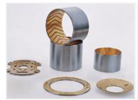
TE80 bimetallic bearing is made of steel sintered with CuPb10Sn10 or CuSn6Zn6Pb3 as a lining layer. In this product range, this type of bushing demonstrates the best performance among bushings made of Cu-lead alloy material. It is well suited for low speeds and high impact conditions. Its usages include balance suspensions of heavy-duty trucks, track roll of bulldozers, car chassis etc.
