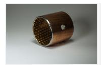
TE93 type lead-free bimetallic bearing, with low carbon steel as base material, which is sintered with CuSn6.5P0.1 alloy layer. It has excellent wear, load and sliding performance. In many operating conditions, bimetal bushings can replaced the lead or bronze bushings.
