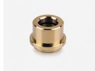
TEJDB01C bearing is made of aluminium brass with graphite embedded in a ring groove. With frictional heat graphite and avle form a metastatic film, which will reduce the friction coefficient and increase operating life.
